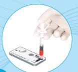
Fill the inlet with sample and cover the cap to seal the sample inlet.
