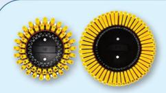
100 reagent positions (R1, R2), double reagent disk positions 24 hour non-stop refrigeration (2-8°c)
