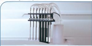
Adopt 8 channels automatic washing mode, wash cuvettes automatically, auto zero setting & deduct/record blank value for each cuvette. More washing times for cuvette of high pollution items to ensure clean thoroughly.
